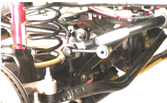
Image 2. Swaybar Link Detached
