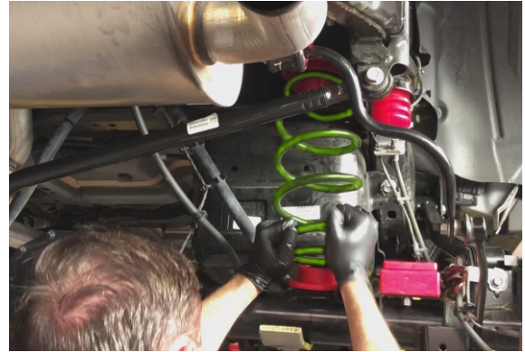
Image 9. Rear Spring Installation
