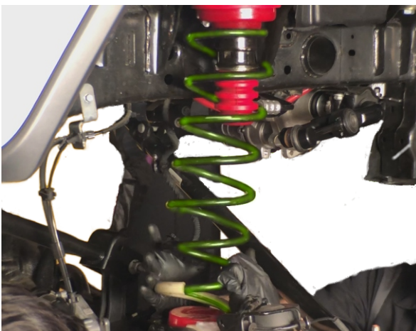
Image 6. Coil Spring Installation
